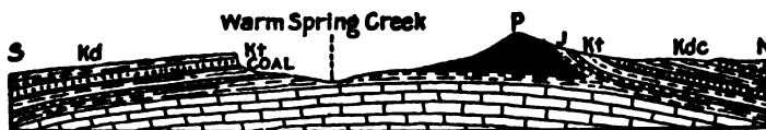
FIG. 13.—Section of Warm Spring laccolith, Montana, showing erosion of roof and of laccolith more advanced than that at Burnett Creek. (Same ref. as for Fig. 10, p. 519.) Solid black , porphyry of laccolith; Kd , Dakota sandstone; Kt , Kootanie sandstone; J , Jurassic; Kdc , Dakota and Colorado groups.
